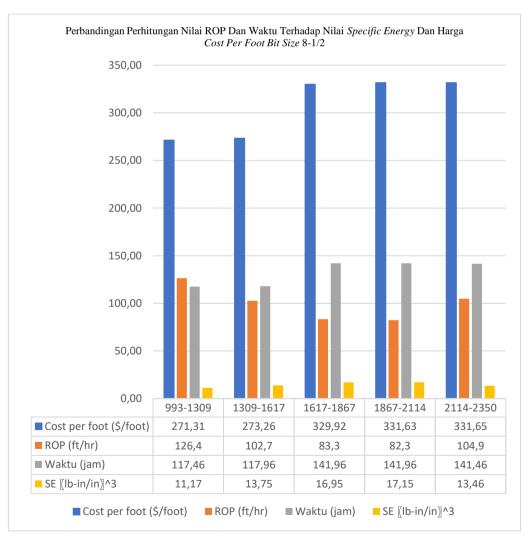
Gambar 6. Perbandingan Perhitungan Nilai ROP Dan Waktu Terhadap Nilai Specific Energy Dan Harga Cros Per Foot Bit Size 18-1/2
