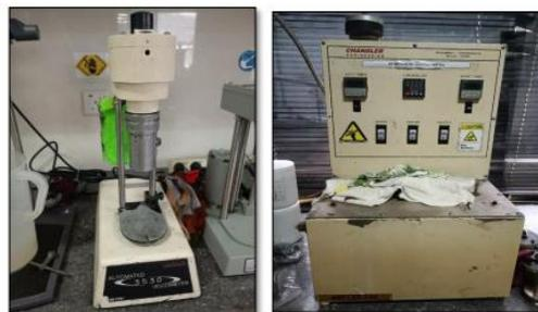
Gambar 1. Alat *Viscometer* dan *atmospheric consistometer*
