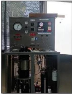
Gambar 3. Gambar HPHT Consistometer
