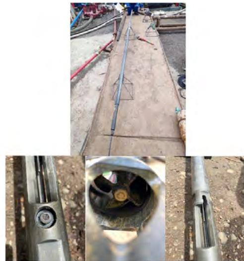
Gambar 2. Rangkaian PTS (Pressure Temperature Spinner).
