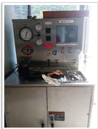
Gambar 2. Alat HPHT Consistometer CTE 22-400
