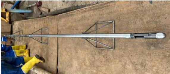
Gambar 1. Rangkaian PT Dummy Logging.
